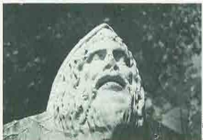
Sulphuric acid in rain eats away marble in Halifax and limestone in Ottawa, where projecting resin provides clue.
