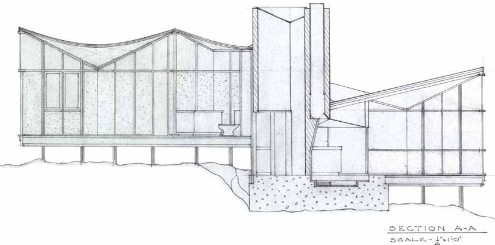
Throughout the home's interior the warm wood overhead that blankets every room is never overwhelming, but reinforces the sense of being in a natural environment. The repetitive lines in this first known central Canadian example of wooden hyperbolic paraboloid pull your gaze outward to the large windows and into the surrounding nature.
